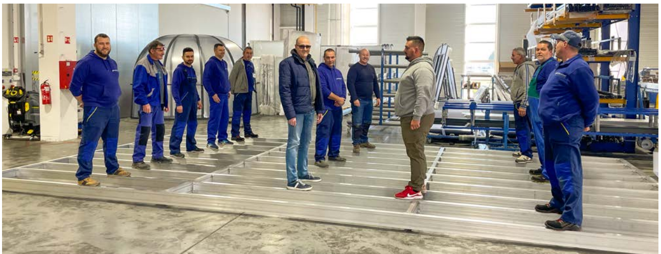
Load test on a pool deck with 8,5 m span
