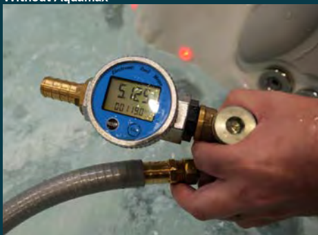
5.125 Liters/min - Standard jets. Test conducted on the Orion Spa
