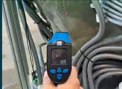
Outside temperature of the tub: 18.9°C Optimal insulation; 17°C difference!
